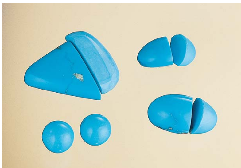
Figure 11. An oxalic acid solution can be used to detect some of the Zachery-treated turquoise. For each pair, the sample on the right was immersed in oxalic acid for four hours. Shown clockwise from the lower left, the samples are: untreated (beads); treated throughout and left natural color; treated throughout and then color treated; and color treated only. Photo by Maha DeMaggio.
